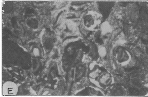
PLATE IV-E. Intra-sparrudite shows clusters of ooids and pellets occurring in intraclastic rock fragments and standing in the sea of sparry calcite as islands. When leached, the porosity becomes very high. Note that sparry calcite recrystallization is more prominent in the oolites than in the pellets and micrite, \times 20 .
