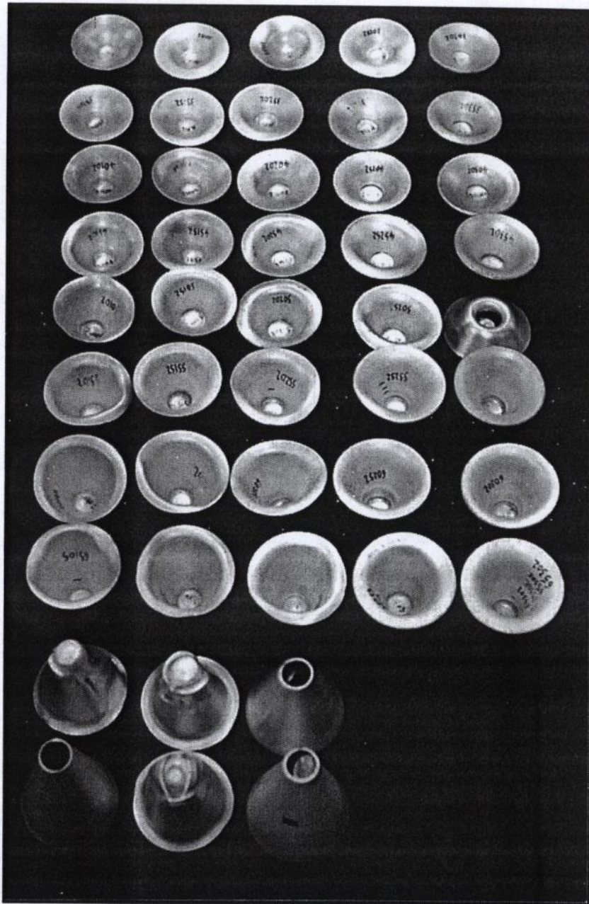
Fig. 2. Spun aluminum specimens after the first inversion.
