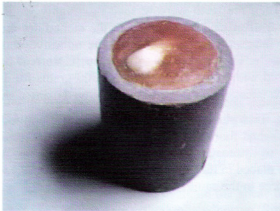
Figure 1: Tooth invested into metal ring using self-curing acrylic resin
